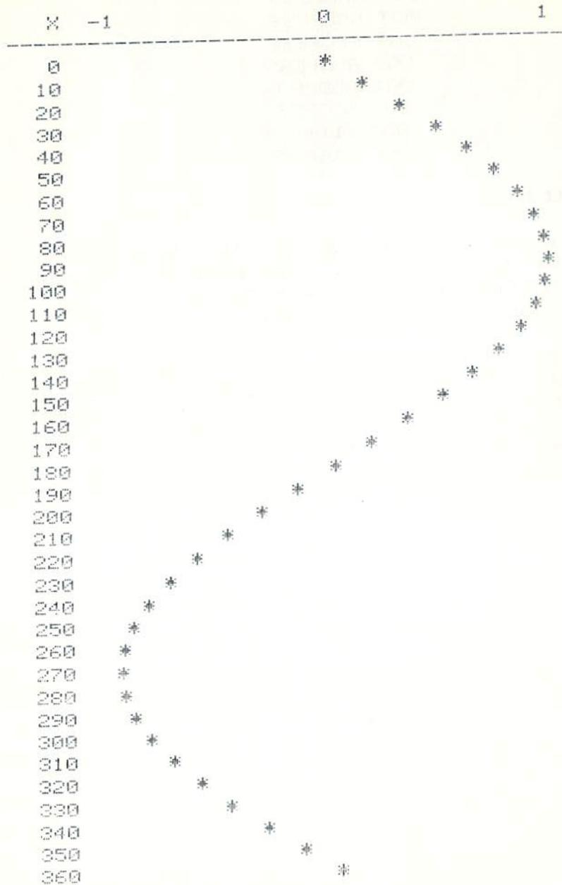
To perform the diagnostic print test, simply turn off the printer, then turn it back on while pressing the Paper Advance Switch.
