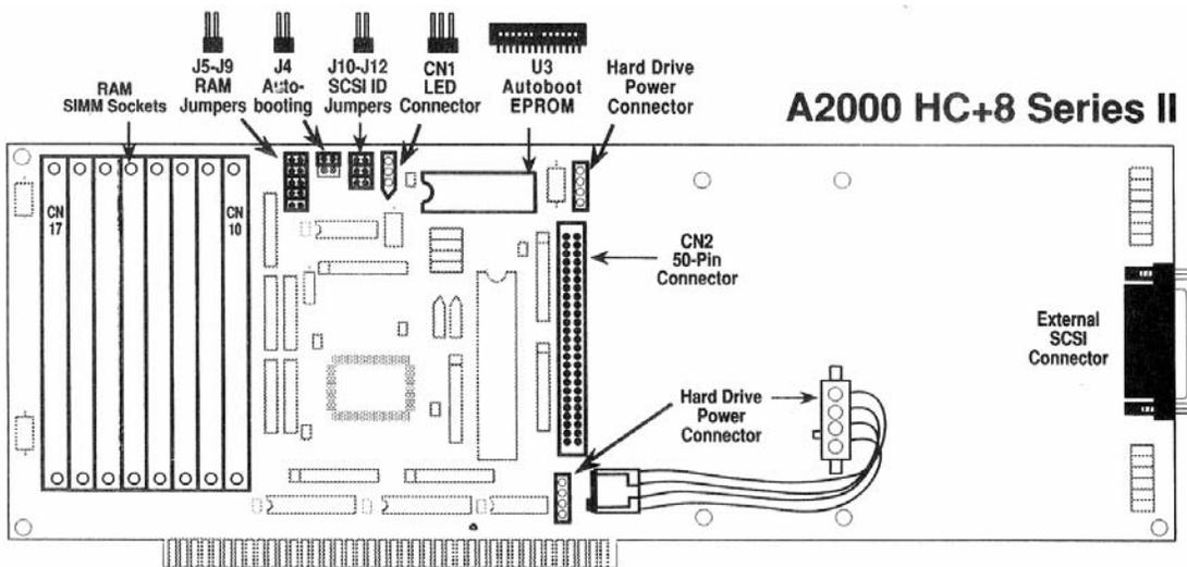
The first step is to determine which product you are going to install and which options, if any, you are going to utilize. The reason for this is that you should perform the installation in a specific order, so that the installation is as simple as possible. The following is a good guideline to use when installing any of the GVP Impact Series II products:
