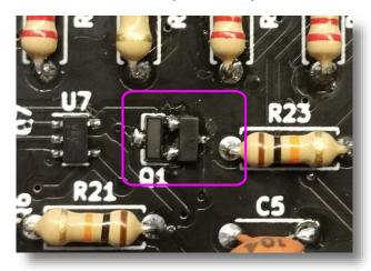
3. Add a wire from the third pin of the new transistor, to the lowest pad of Q7.
