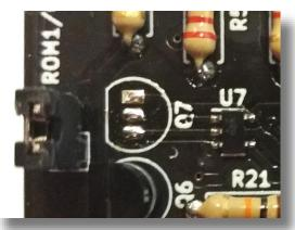
2. Solder the new transistor *upside down* to Q1 - you can solder both joints from the sides. We marked the *top* of BSS84 with silver paint, so you should *not* see that.
