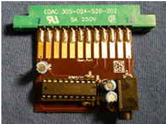
If the beautiful analogue sound of the SID chip isn't suitable, maybe it's time to go digital instead? For this, we've created the DigiMAX. When plugged into your User Port, it provides four 8-bit digital sound channels (in stereo) through a separate output on the card. With appropriate cables and mixer (not included), one can even use the SID and DigiMAX together.
